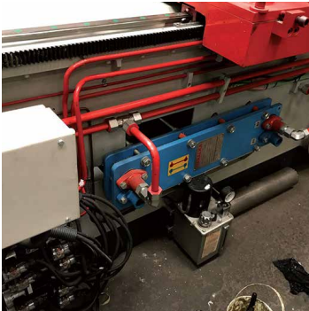
Oil Cooling in an Special Purpose Machine
